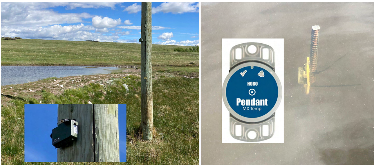
Figure 2. Song Meter sound recorder and Hobo Pendant water temperature recorder deployed at the Pennask Lake Road PEN13 pond. This site produced high-quality Spadefoot recordings and was selected for the preliminary analysis reported here.
